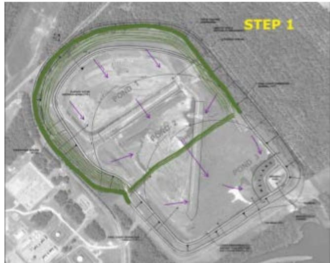
A geomembrane option (GCL or 30-mil FML) is the preferred long-term remedy for areas with groundwater impacts. The top of the disposal unit can be lined and capped for a developable plateau.
