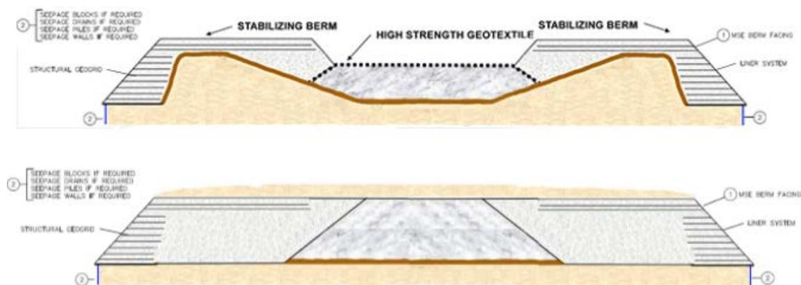
The AWT berm system is a Subtitle D-compliant lined approach that complies with EPA regulation and addresses state regulatory programs. A geomembrane option (GCL or 30-mil FML) is the preferred long-term remedy for areas with groundwater impacts. The berm can be constructed 50 to 75 feet inside of the current CCR waste boundary to allow for future groundwater control methods.
